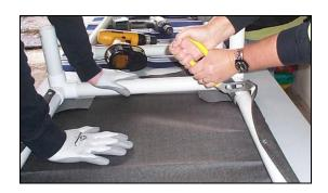
Screw one screw to the opposite side of the frame, then use channel locks to tighten frame. This will tighten the cloth.
