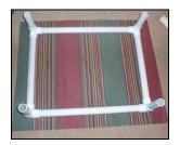
4 Lay cloth on a flat surface and lay the frame on top of cloth, with legs pointing up. Center the frame on the cloth.
