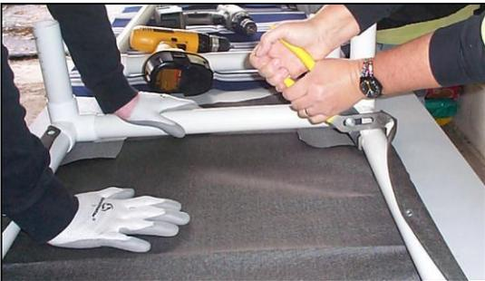
**9** Screw one screw to the opposite side of the frame, then use channel locks to tighten frame. This will tighten the cloth.
